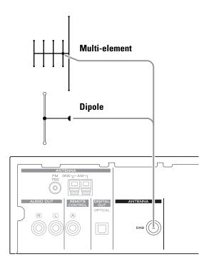
It is possible to use a TV or FM antenna with your DAB tuner as this is normally mounted externally.
